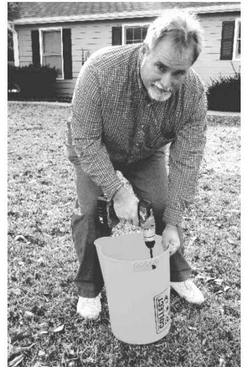
Collector tube extends up from bottom of bucket. To collect soil sample, the operator runs a cordless drill-powered auger through tube and into the ground.
