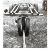
it anywhere. The tandem dual wheels pull through mud without sinking and the front wheels turn 360 degrees like a big castor wheel so I never get stuck."
