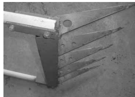
Teeth look like angled steel "chisels" and easily slice through compacted ground.
