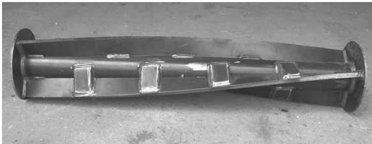
Rock beater has a spiral shape, which ensures that 70 percent of the opening in the beater is always open so crop can flow smoothly into rotor.
