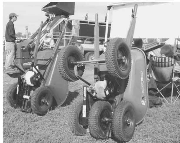
Photo shows 2-wheel-drive model, left, and 3-wheel-drive model, which is also fitted with optional rear wheel kit.
