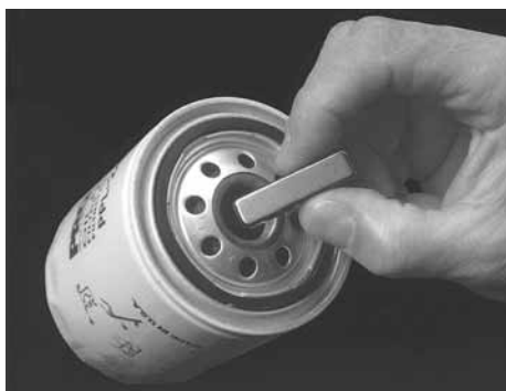
Magnet catches particles too small for an oil filter to stop. It's designed to be dropped into the center hole of any spin-on oil filter with a metal core.
