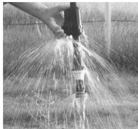
Filter fits between the hose and the regulator on center pivot drop nozzles (left). To flush out sediment you just push up a small release valve on side of filter.
