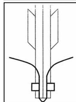
**Wild Chance Post Anchor attaches to any steel post with a pair of pliers. As post is pulled upward, wings bow out to hold it in place.**
