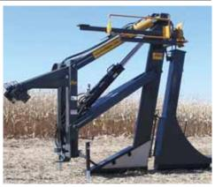
Interchangeable boots mount on quick-tach tile plow by simply pulling a single rod.
