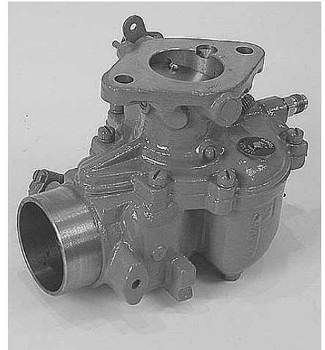
Gary Hoefling says his modified Zenith carburetor cleans up the black smoke and fouled spark plugs common to Deere 3010/3020 and 4010/4020 tractors.
