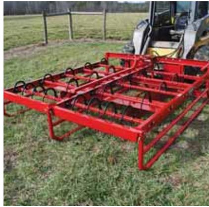
Loader-mounted “Accumagrapple” gathers up 8 to 10 small square bales in the field. Once the bales are gathered together, they can be loaded onto a truck or trailer, with the same piece of equipment.
