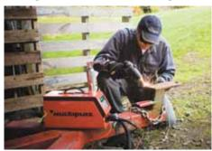
Not much bigger than an old-time radio, all the Multiplaz 3500 welder needs is 110 or 220-volt current, water and alcohol.
