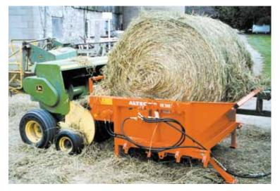
doesn't break up the hay but instead gently unwinds it. The legs are needed only if the baler's pickup reel is more than 2 ft. off the ground. And when you're done using the unwinder to make small square bales, you can remove the legs and use it as a normal bale unwinder to deliver feed into bunks or onto pasture ground."
