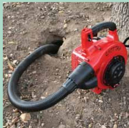
**Gas-powered Cheetah uses a small engine and fan to push exhaust fumes into pest tunnels.**
