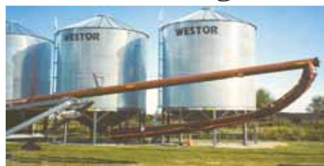
**The 30-ft. flexible spout extension makes it easier to fill grain bagger with an auger and semi truck, instead of having to use a smaller grain cart or tandem axle truck.**
