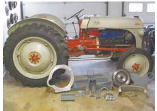
**Photo shows parts included in overhead valve conversion kit for N-Series Fords.**
