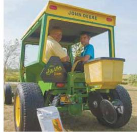
Gene Brass's green and yellow hot rod looks like a Deere tractor but can cruise at road speeds up to 80 mph. Quick-tach hitch on back of cab supports a 1-row planter unit.
