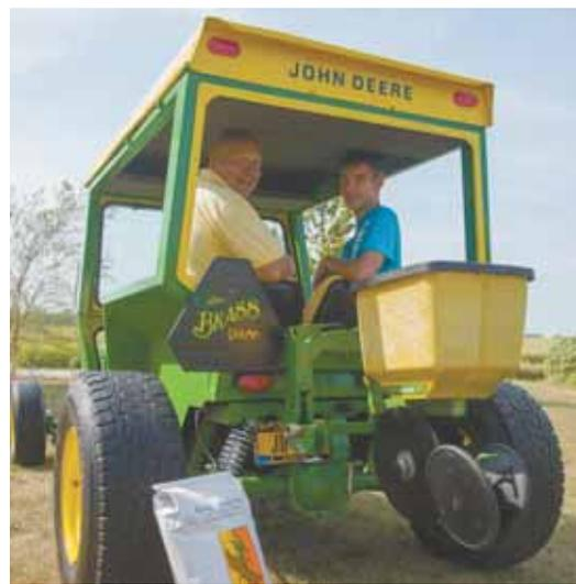
Gene Brass's green and yellow hot rod looks like a Deere tractor but can cruise at road speeds up to 80 mph. Quick-tach hitch on back of cab supports a 1-row planter unit.
