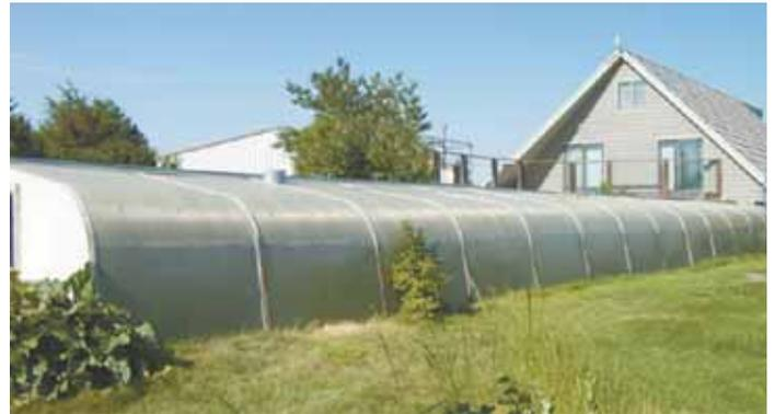
“Underground” greenhouse is buried 5 ft. below ground and measures 80 ft. long by 16 ft. wide. It uses earth heat as the only source of heating and cooling.
