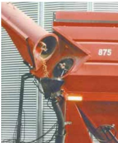
Grain spilling out of folded-down auger falls into boot and is held in a piece of drain tile below.
