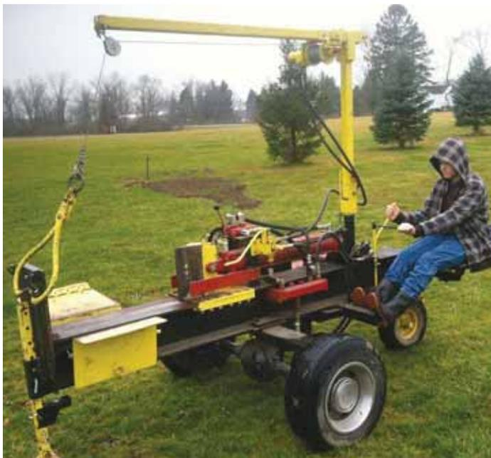
Andrew Youngblood's 3-wheeled, self-propelled splitter is equipped with a crane fitted with tongs, which are used to lift heavy chunks onto the splitter table.
