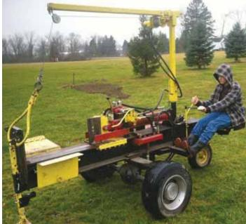
Andrew Youngblood's 3-wheeled, self-propelled splitter is equipped with a crane fitted with tongs, which are used to lift heavy chunks onto the splitter table.
