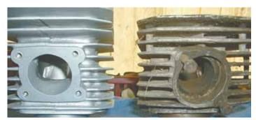
Bead blaster uses no. 80 glass beads to remove rust, oxidation and corrosion without damaging metal parts.
