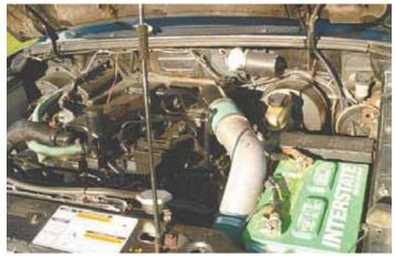
Jacob Kraybill repowered this Ford Ranger with a Cummins 3.3L industrial engine, building an adapter ring to connect the diesel flywheel with the flywheel from the Ranger's original gas engine.
