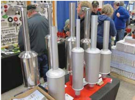
“Restoration quality” mufflers for Farmalls are available in both aluminized steel and polished stainless steel.
