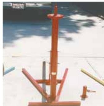
After the bead is broken, Terry lifts wheel up and puts it on flange at top of post to pull tire off rim.
