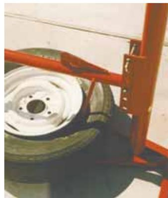
A lever slips between the rim and the tire. By pushing a handle down, the lever breaks the tire’s seal.
