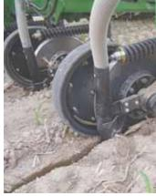
Fertilizer is precisely placed 2 in. to the side and 2 in. below the seed.
