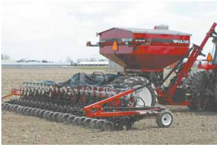
Aulari offers this tow-between cart equipped with a universal hitch that matches different types of equipment.
