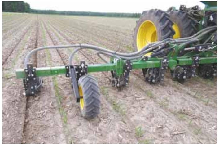
The company offers precision placement fertilizer coulters for side dressing granular fertilizer.
