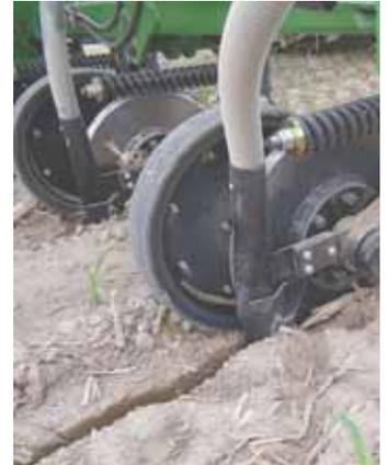
Fertilizer is precisely placed 2 in. to the side and 2 in. below the seed.
