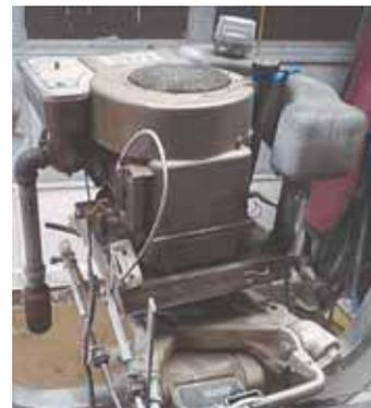
Al Smith repowered an old boat with the 11 hp Briggs & Stratton motor off an old riding mower.
