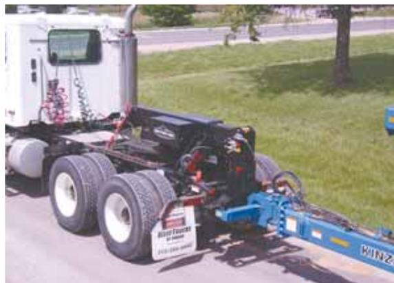
If you don't have a tractor handy, you can use a semi-tractor to shuttle big equipment by adding a Retriever hitch on back.
