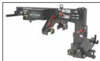
Hitch lift mast mounts securely to semi-tractor's fifth wheel receiver with a plate and kingpin.
