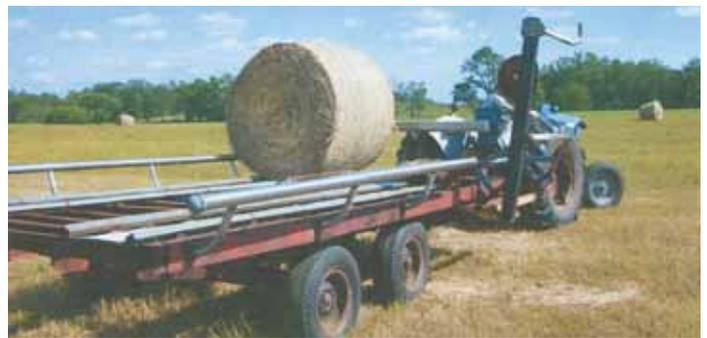
**Bill Ranallo built this self-loading round bale hauler out of an old pull-type pea viner. Once all 8 bales are loaded, the operator tips bales off the back.**
