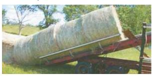
Machine is equipped with a pair of ĥvdraulicoperated forks on front, as well as a push plate that moves bales back 2 at a time.
