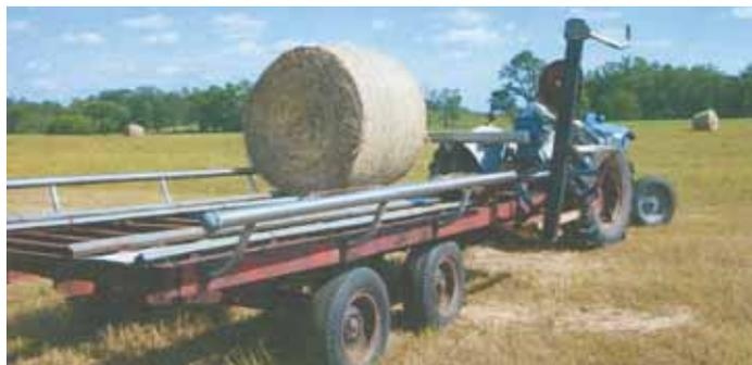
**Bill Ranallo built this self-loading round bale hauler out of an old pull-type pea viner. Once all 8 bales are loaded, the operator tips bales off the back.**
