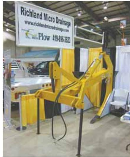
The 3-pt. mounted Richland Micro Plow is designed to lay small 2-in. dia. poly tile only 2 ft. deep. "We find that it's more cost effective to use 2-in. tile on 20-ft. spacings," says inventor Mark Martin.
