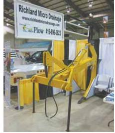
The 3-pt. mounted Richland Micro Plow is designed to lay small 2-in. dia. poly tile only 2 ft. deep. "We find that it's more cost effective to use 2-in. tile on 20-ft. spacings," says inventor Mark Martin.
