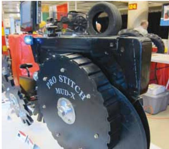
Pro-Stitch Mud-X gauge wheel has molded lugs built into it, which allows it to gain traction even in muddy ground. The gauge wheel also acts as a scraper, keeping the disc opener clean.
