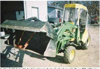
LaVier Schliefert added a hinged top to the loader bucket on his Deere 855 utility tractor. A welded-on grader blade forms the top's cutting edge.
