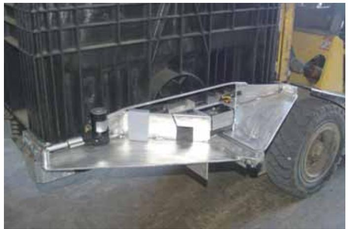
Seed box opening system comes with an aluminum frame that's held to box by means of an electric actuator. Another actuator is used to open and close box's slide gate.
