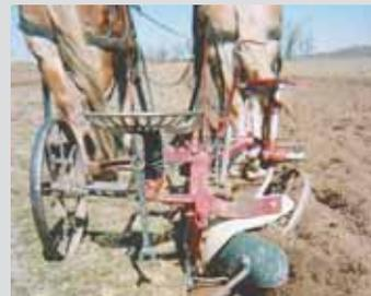
Floyd Sumy needed a new plow share for his Oliver 40 sulky, 12-in. bottom plow, so he cut down an old 16-in. IH moldboard to fit.
