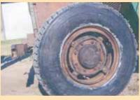
He replaced the front assist wheels on the tractor with truck wheels and tubeless tires, using 10-22.5 retread tires mounted on open center wheels. He made an adapter plate from 5/16-in. thick plates, with four ear mounts for the truck wheel on it.
