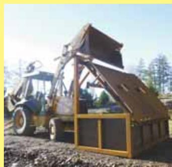
A front-end loader is used to dump the load over an angled screen.
