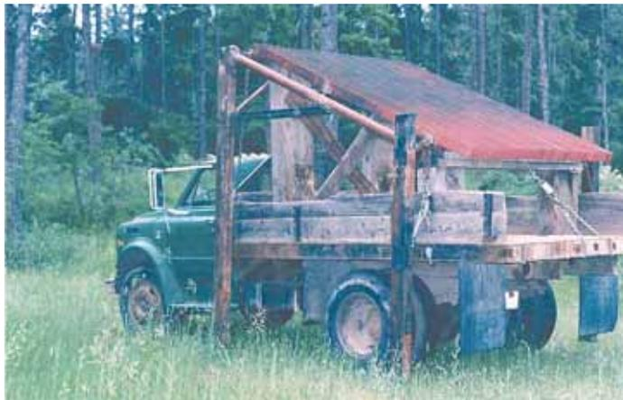
Ross Wilkinson converted the intake grate from a hydroelectric dam into this gravel screen, mounting it on an upright steel frame that he can back a truck under.
