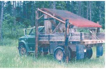
Ross Wilkinson converted the intake grate from a hydroelectric dam into this gravel screen, mounting it on an upright steel frame that he can back a truck under.
