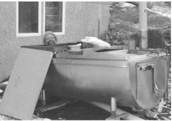
Del Stubbs converted an old 250-gal. milk tank into a low-cost hot tub. He removed tank's top doors and installed a submersible wood-burning heater at one end.
