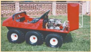
Home-built, all-wheel-drive 6-wheeler has an all-steel body and rides on six 30-in. high, 10-in. wide wheels.
