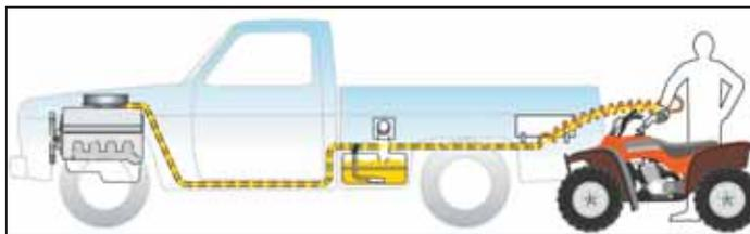
**Fuel transfer system turns your pickup's fuel tank into a mobile gas station. A flexible hose and nozzle reach 5 ft. beyond pickup and are protected in an aluminum container when not in use.**
