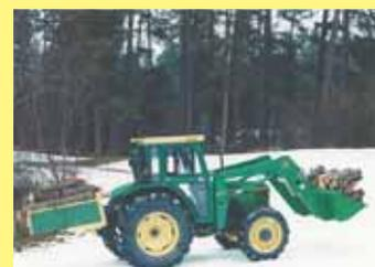
**Ross Wilkinson built a full line of equipment for his Deere loader tractor, including a flexible blade (above left), log forks that fit inside a conventional bucket (above right), an extra-wide pallet fork (lower left), and 3-pt. mounted box.**
