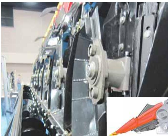
Photo shows underside of new cornhead. Wind generating blades chop stalks into 4 to 18-in. pieces, then blow them horizontally into an auger. It delivers the material to middle of header, forming a windrow. Inset drawing shows auger under header.
