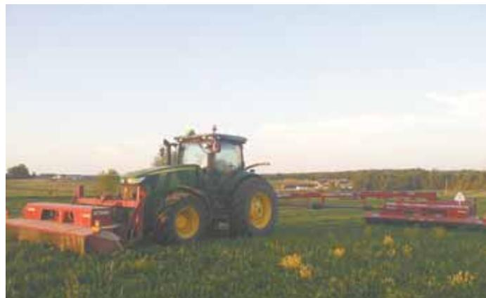
Willie Albrecht modified a new New Holland 7560 haybine to mount on front of his 300 hp tractor. A second haybine cuts off to the side to create a 30-ft. swath.
