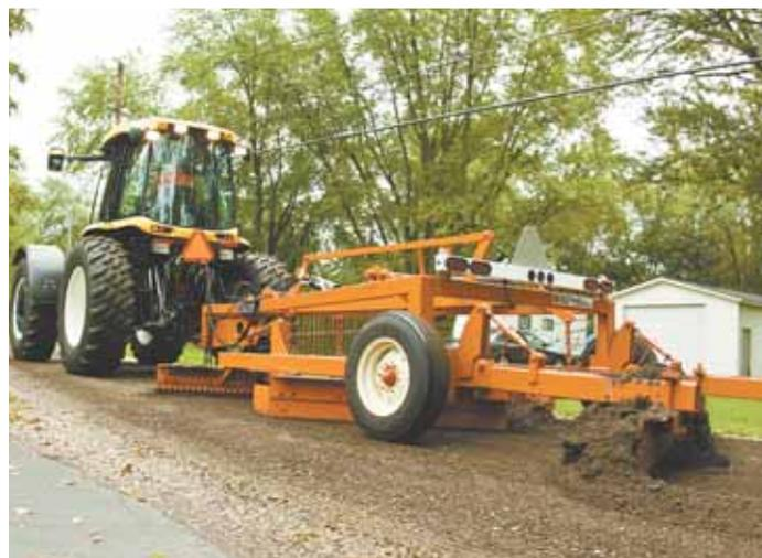
Bonnell Industries says its pull-type Road Maintainer can do everything a self-propelled road grader can do, for a fraction of the price.
