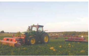
Willie Albrecht modified a new New Holland 7560 haybine to mount on front of his 300 hp tractor. A second haybine cuts off to the side to create a 30-ft. swath.
