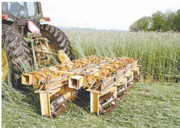
Modified stalk chopper makes fast work of heavy cover crops, crimping and pushing them down in a solid mat.
