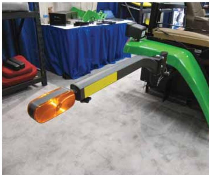
**Tractor or combine-mounted warning light consists of a telescoping metal bar with reflective tape on both sides, and a large amber light at one end.**
