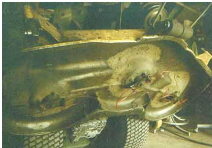
**LaVier Schliefert can convert his riding mower into a giant "weed eater" by replacing the blades with heavy-duty weed eater strings.**
