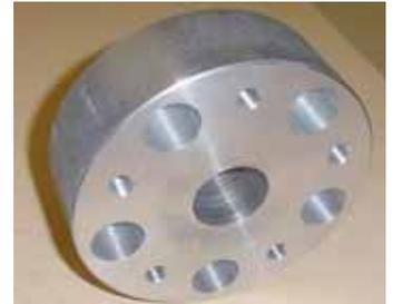
Wheel's original bolts are used to bolt wheel rim to spacer.
