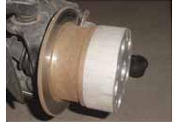
The 6-in. dia. solid aluminum wheel spacers come with hardware to bolt to the Gator's wheel hub.
