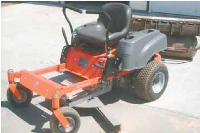
Richard Gostomski built this 5-ft. wide, belly-mounted grader for his Husqvarna zero turn riding mower. Grader blade mounts in place of the mower deck.
