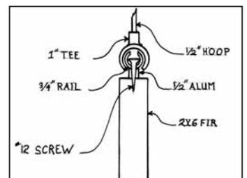
Multiple hoops glide on rails, making access to the garden bed as easy as pulling on two ropes.
