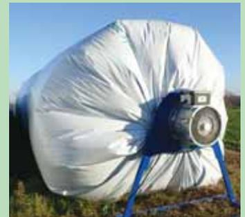
Bales are loaded into one end of bag using a specially designed, square bagging frame (upper left). A large fan blows air into bags, (above). The finished end of the bag is closed to the desired diameter to control air flow.
