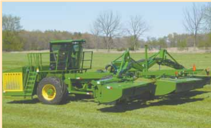
Self-propelled, mower conditioner is equipped with three 16-ft. cutting and conditioning heads.
