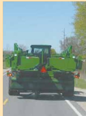
The 3 mower heads are tucked into a 15-ft. width behind cab during transport.
