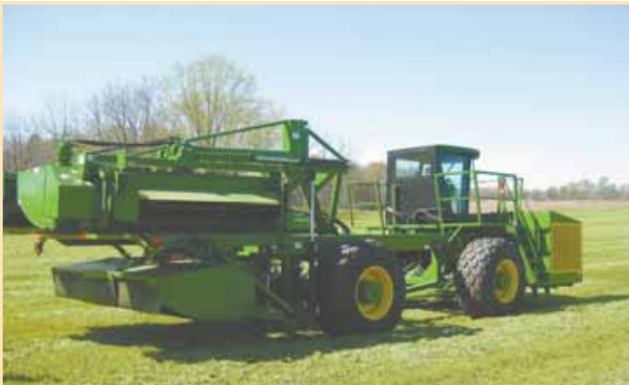
Machine's Deere cab mounts on a manual turntable, allowing the operator to drive forward both in the field and on the road. Cab can be turned 180 degrees for transport.
