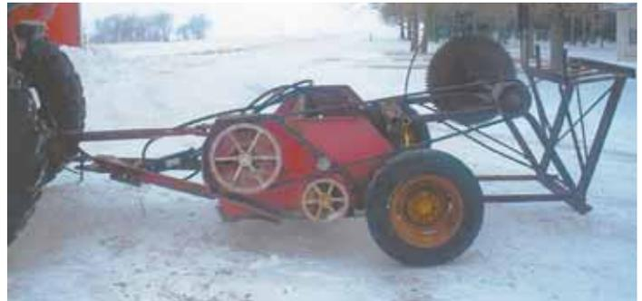
David Schmidt converted a saw arbor and an old pull-type forage chopper into this pto-driven buzz saw.
