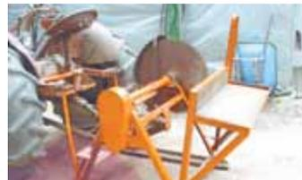
Don Ramberg converted the flat belt drive on his front-mounted buzz saw to a 3-pt. mounted, pto-drive unit.
