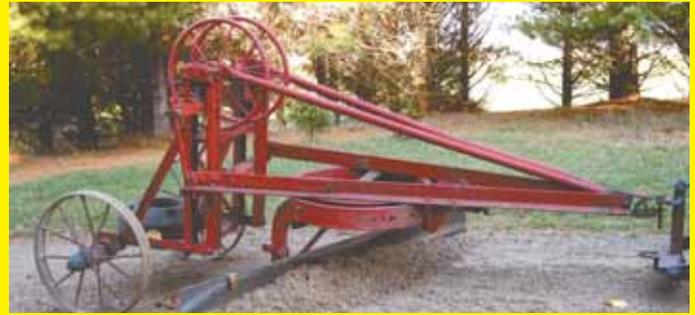
I use an old horse-drawn grader to level my long gravel driveway. It's pulled from the 3-pt. hitch, which allows me to precisely control the grade. I made a new one for a friend that tilts and
