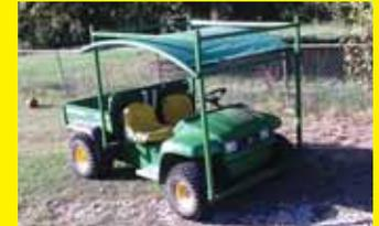
I used 1 1/2-in. sq. tubing to build this "Gator topper" for some friends in Texas. It's equipped with a "half moon" top made from a section of trampoline framing that's covered with canvas. My friends asked me to extend the frame upward so they could transport their 2 kayaks to a pond 1/4 mile from their house, so I did.
