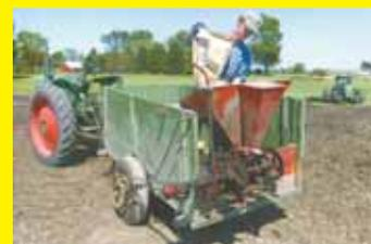
We use an old ground-driven endgate seeder to broadcast seed onto the ground. We mounted a 40-bu. wagon box on an old car axle and a V-shaped metal frame. We also bolted a big sprocket to
