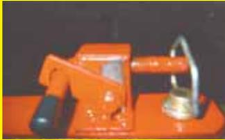
Here's a solution to the problem of lost hitch pins that come out. This "hitchkeeper" welds to the top of the implement hitch. Just flip the locking device down over the hitch pin and it's locked. You'll never lose another pin. (Harold Fratzke, Cottonwood, Minn.)
