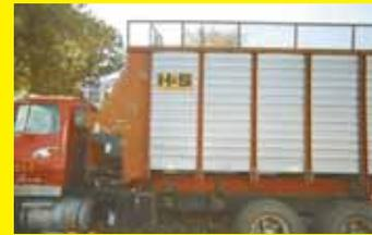
We recently mounted an old H&S self-unloading, 18-ft. wagon box on a tandem axle truck for a local dairy farmer who uses it to haul hay and corn silage. He has fields scattered several miles apart, and with the truck, he can drive down the road faster between fields.
