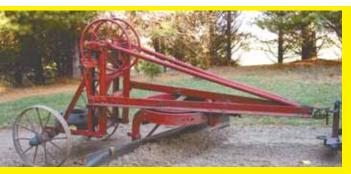
I use an old horse-drawn grader to level my long gravel driveway. It's pulled from the 3-pt. hitch, which allows me to precisely control the grade. I made a new one for a friend that tilts and swivels like this one, but has rubber tires. (Gerald Johnston, 5821 Crystal Rd., Vestaburg, Mich. 48891, ph 989 268-5650)
